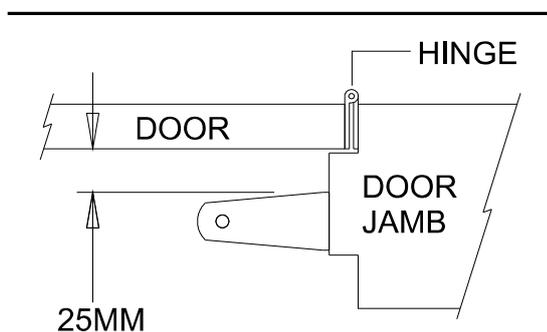
**1** Place the **Jamb Bracket** on the hinged side of the door jamb, 25mm from the face of the door and 40mm down from the top of the door. Fasten the **Jamb Bracket** with the three **25mm screws** provided.
