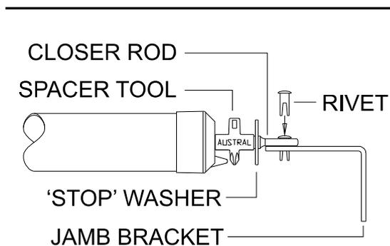
**2** Place the **Stop Washer** over the **Rod** and place the **Rod** onto the **Jamb Bracket**. Slip the forked **Rivet** supplied through both. **Do not** deform the legs of the **Rivet** or remove the **Spacer Tool** at this stage.
