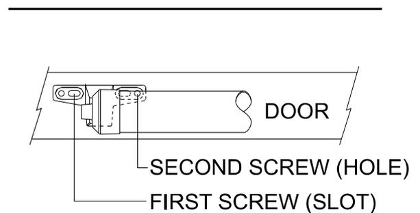
**4** Mark the centre of the first screw slot and drill a 3mm hole at this mark. Fasten the **Door Bracket** with one **12mm Screw**. Remove the **Closer** (jamb end first) and drill through the second screw hole. Fit the second **12mm Screw** in the **Door Bracket** and refit the **Closer**.
