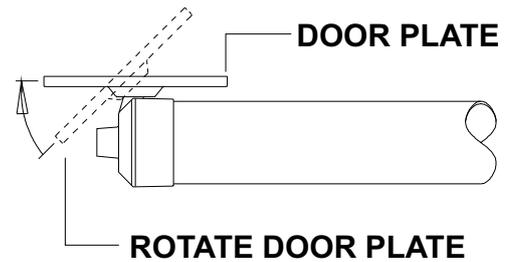
**3** Fit the **Door Plate** onto the **Closer Foot** as shown above. With the door fully closed and the latch engaged, swing the **Closer** and **Door Plate** onto the door in a level position
