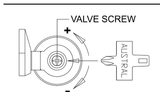
**5** Open the door, remove the **Spacer Tool** from the **Closer Rod**. Test the **Closer** and adjust the **Valve Screw** with **Spacer Tool** to control the closer speed. Deform the **Rivet** with the back of the **Spacer Tool**.
