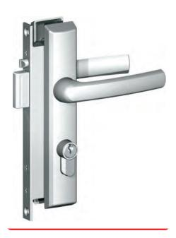
**Operation:** A reliable mortise lock for hinged doors having a latch bolt that is retracted by operation of either an outside or inside lever. Closing the door causes an auxiliary bolt to release the latch bolt enabling it to enter the aperture in a strike plate. Once fully extended it may be locked (or unlocked) from either side by key.
