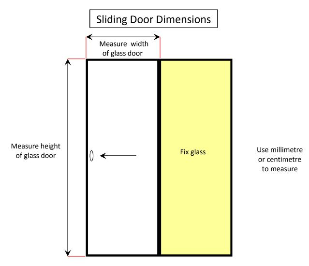
Take dimensions of moving glass door width and height and that will also be the dimension of your screen door. Please note these only used for the purpose of quoting only as they are not exact cut sizes dimensions. **Top View**
